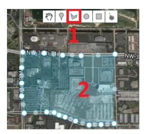
2. To close the Geofence, click on the first point one more time. You will then see your Geofence high-lighted in blue. You can modify the shape of the Geofence by clicking on any of the points lying on the outer edge and dragging them to the desired shape. You can also move the Geofence by clicking in the center of the Geofence, and dragging it.
