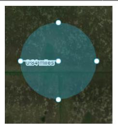
1. Click the circular Geofence button at the top of the map. Your cursor will now change to a + symbol. Click where you would like the center of your Geofence to be and drag the cursor until your Geofence is the desired size. Once your Geofence is the correct size, click again. To move the Geofence, click in the middle of the circle and drag it to the desired location.
